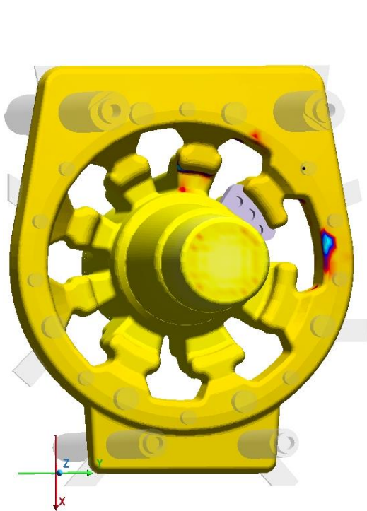
v03_d2 Core Shooting, Sand Fraction 2.000s X-Ray: on
