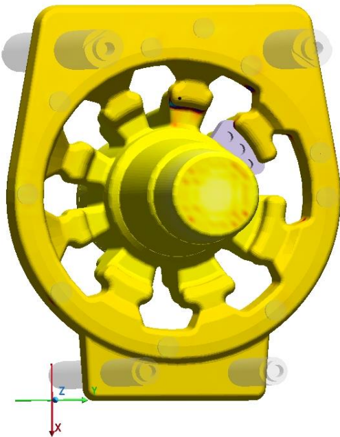
v06 Core Shooting, Sand Fraction 2.000s X-Ray: on
