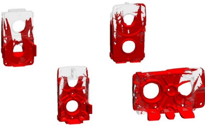
Figure 10 Simulation flow front comparison for 4 possible positionings of the same part, run with MAGMASOFT® version 5.5.
