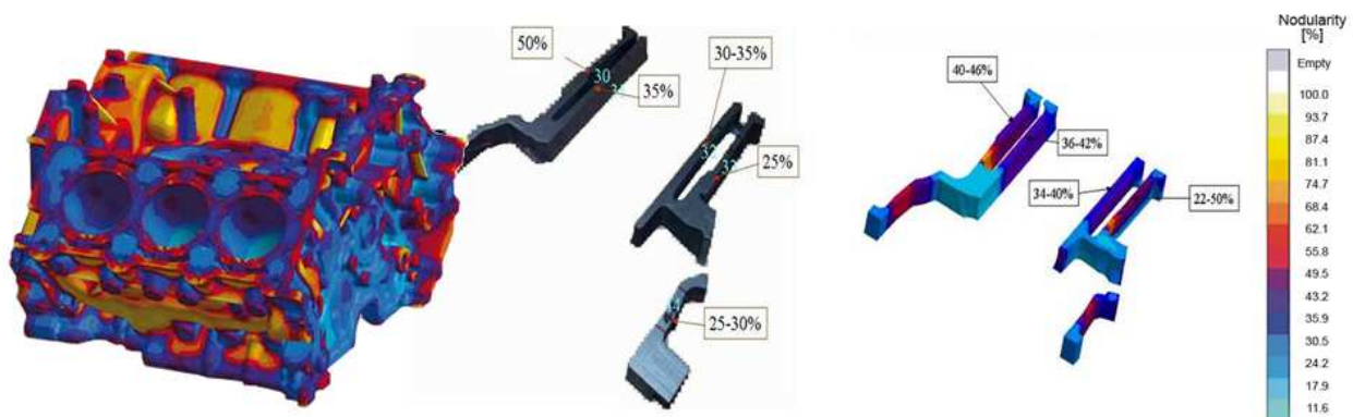
Fig. 9: Simulating local nodularity as a function of alloy, metallurgy, and cooling conditions. Simulated nodularity values are compared with measured nodularity [14, 15].
