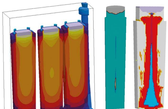
Ingot and mold temperatures in the cluster (left); porosity indications, CET zone (right)
