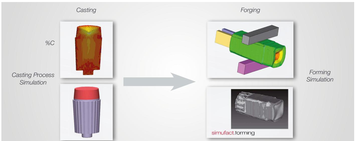
Simulation of the complete process chain – transfer of as-cast properties to forging simulation
