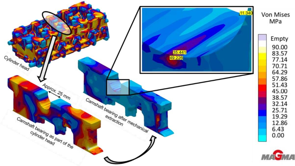
Figure 5: Representation of the simulated Von Mises equivalent stress after T6W heat-treatment of the entire cylinder head (top left), in the camshaft bearing as part of the cylinder head (bottom left) and after mechanical extraction of the camshaft bearing for the validation tests (center)
