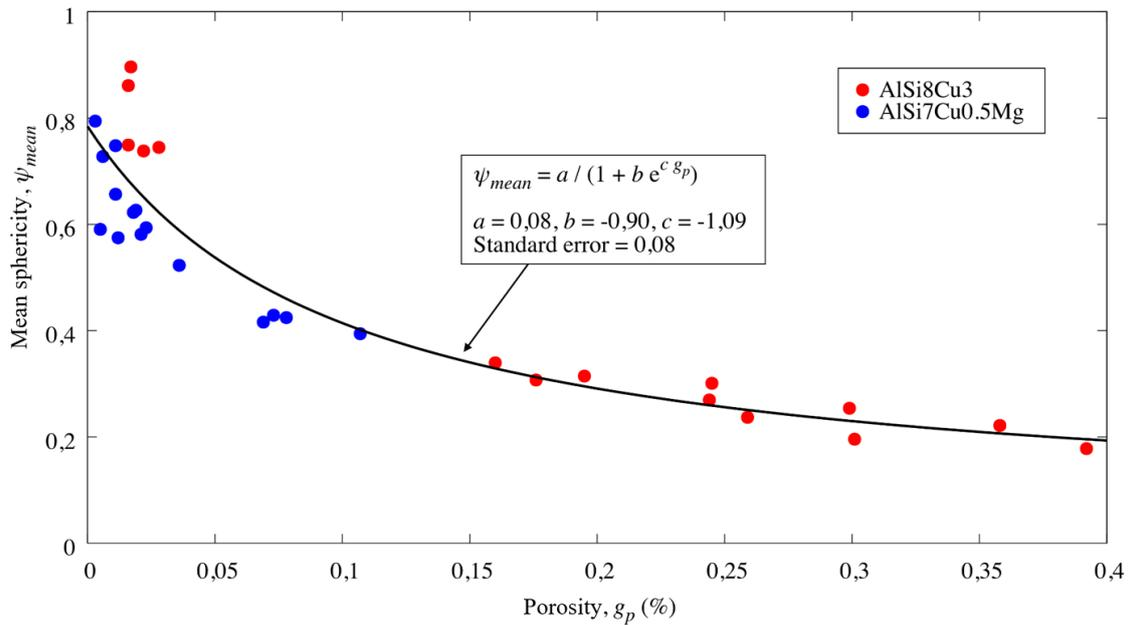
Figure 4: Plot of volume-weighted mean sphericity versus porosity
