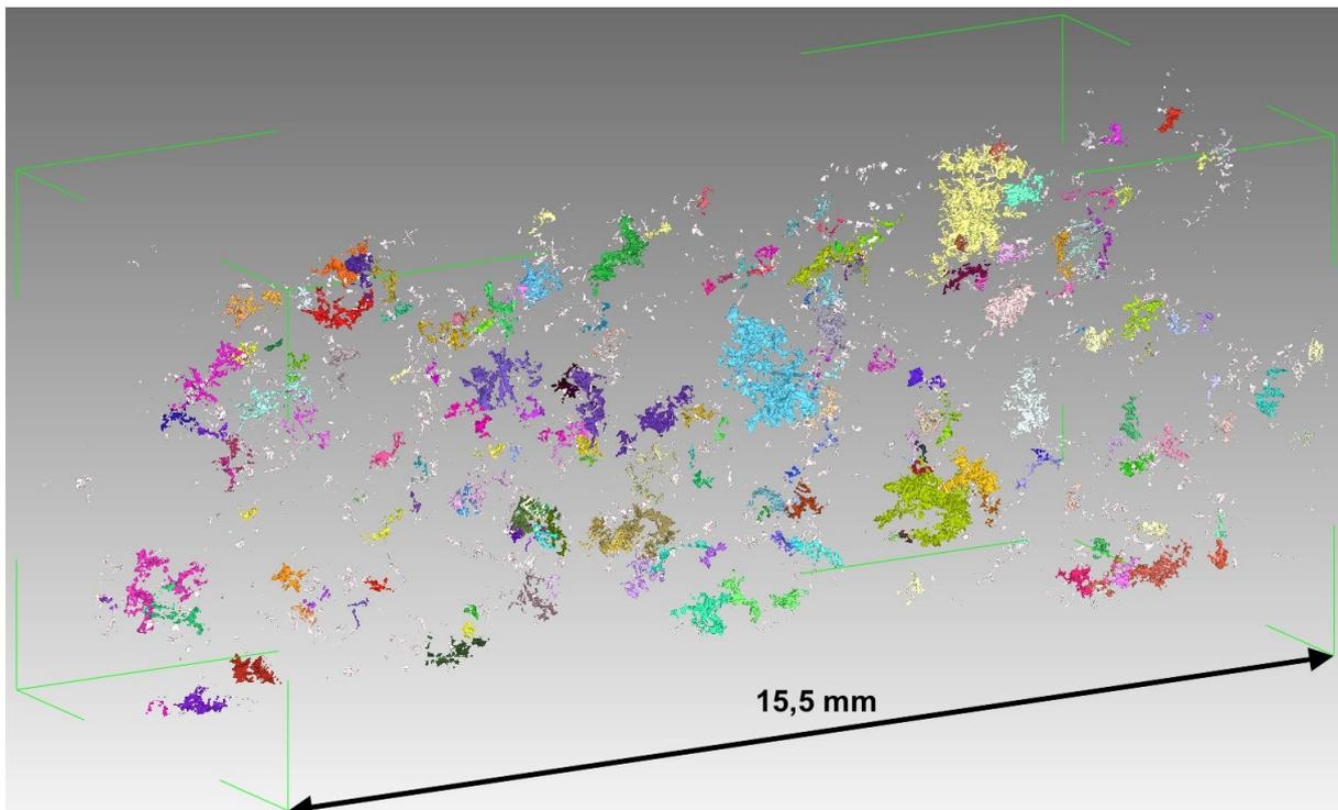
Figure 2: Three-dimensional representation of an XCT sample from the tween deck of an AlSi8Cu3 cylinder head. The porosity is 0.176 %, the maximum diameter of the pore envelope is  $d_{e,max}$  2.75 mm. The coloring of the individual pores is done randomly and serves only for better differentiation of the individual pores [5].
