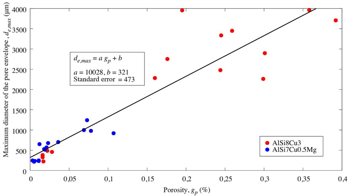
Figure 3: Plot of maximum envelope diameter plotted against porosity [5].
