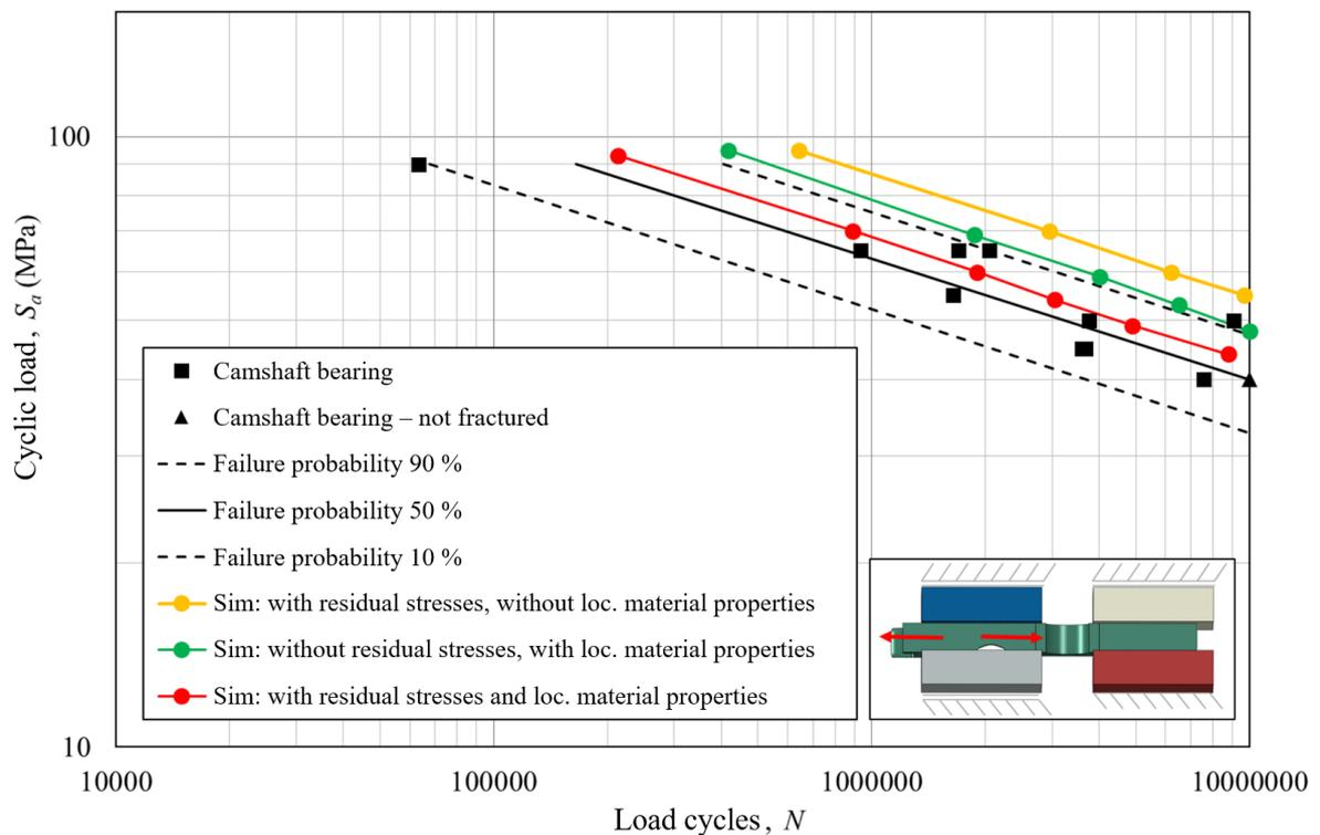
Figure 8: Result of the tension-compressive fatigue test of the cylinder head camshaft bearing samples ( $R = -1$ ) of the alloy  $AlSi7Cu0.5Mg$  (T6W) [13]
