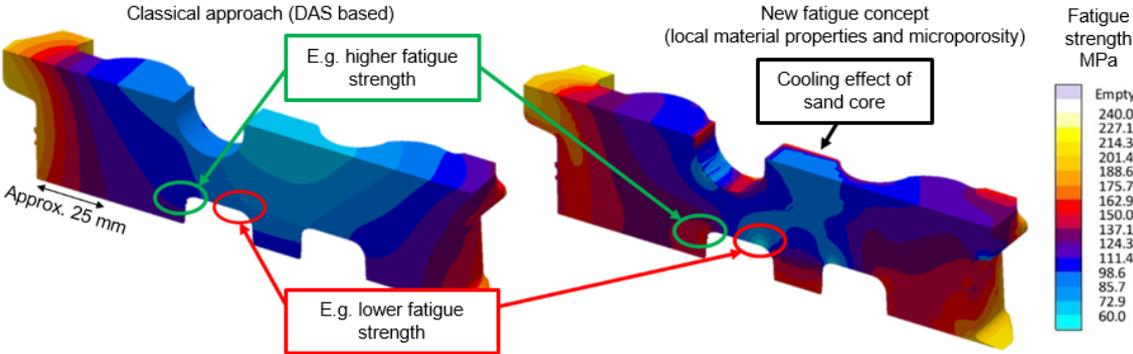
Figure 6: Plot of the tension-compressive fatigue strength in section through the center of the camshaft bearing using the "classical" approach, based on the local DAS (left), as well as based on the additionally included microporosity prediction and the derived defect size (right)
