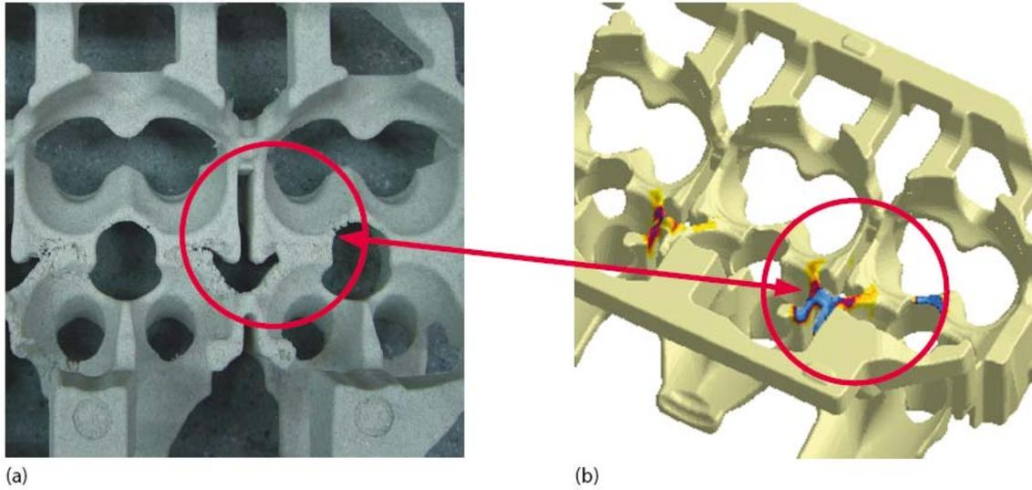
**Fig. 4. Comparison of defects in a water jacket core (a) with respective simulation result (low values of sand fraction are identified in blue) (b).**
