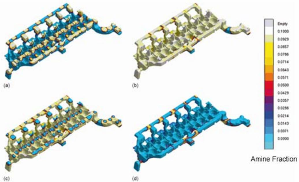
**Fig. 7. Simulation of a two-step gas curing for the PUR-cold-box-process. Initially, a catalyst is introduced into the core, displacing the air previously occupying the porous areas of the core (a, b). Subsequently the amine containing gas is purged by the air pushed into the core (c, d). Amine fraction of 0.1 equals 10% amine.**
