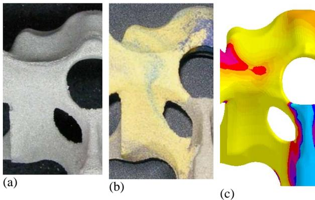
**Fig. 6. Production core (a) and experimental core with colored sand (b) and corresponding simulation result for sand trace (c).**
