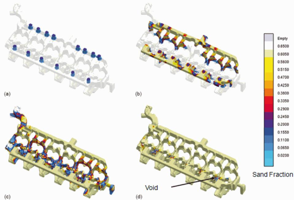
**Fig. 3. Filling sequence for the core shooting process of a thin-walled water jacket core. The sand fraction result is shown for (a) 1%, (b) 25%, (c) 75%, and (d) 100% through the core shooting simulation. Problem areas that contain low sand fraction values are observed at the end of the shooting simulation (d).**
