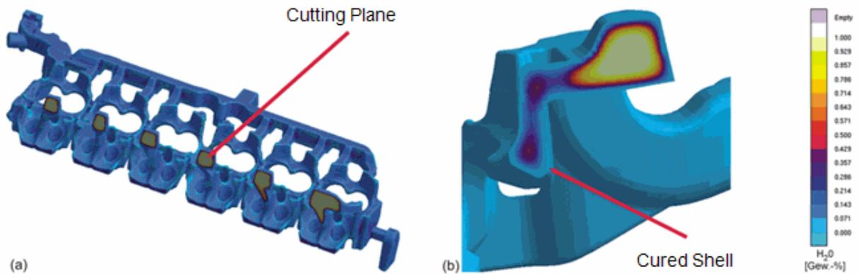
**Fig. 10. Heat curing visualization of entire core (a) and close up of sliced section (b).**
