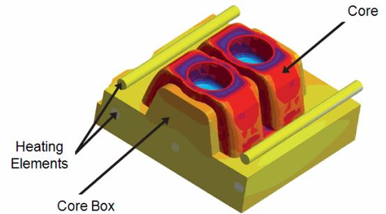
**Fig. 9. Partial view of an electrically heated core box in the heat curing stage.**
