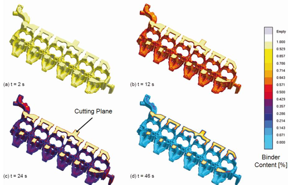
**Fig. 11. Simulation of binder degradation using a starting pouring temperature of 750 C (1382 F).**
