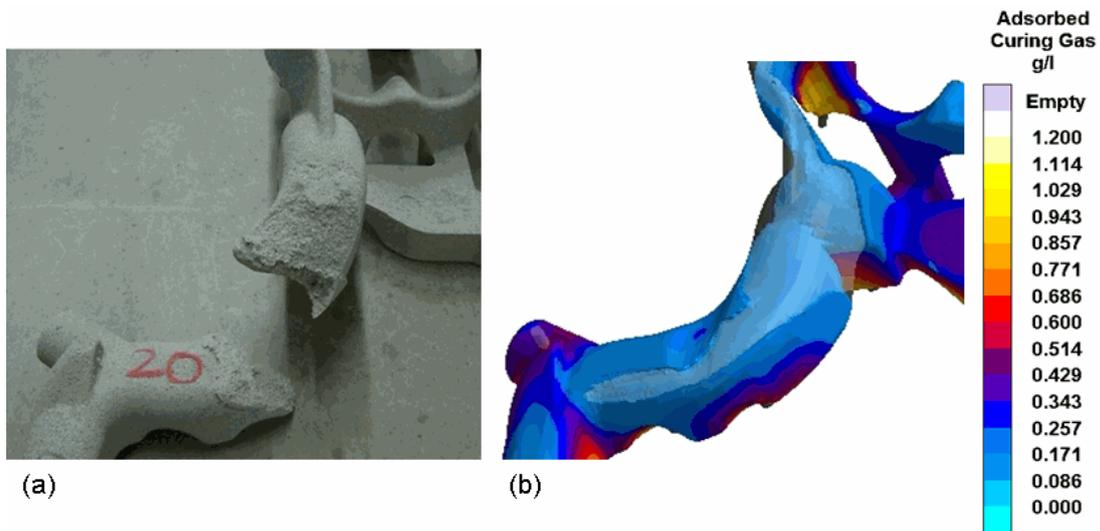
**Fig. 8. Insufficiently cured PUCB core (a) and uncured areas identified by transparent material in the simulation (b).**
