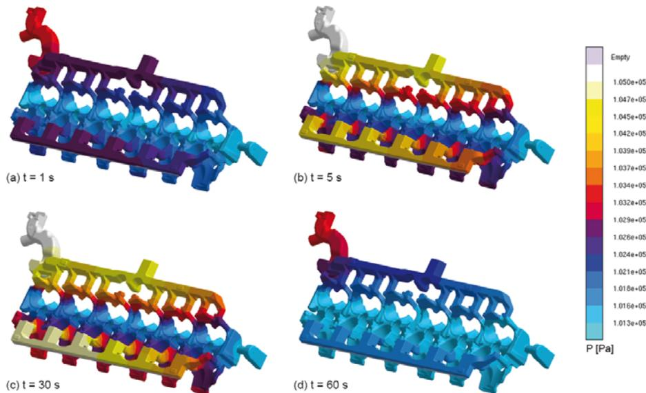
**Fig. 12. Simulation of binder degradation during the casting process, displaying the pressure distribution of a core vented at its central axis.**
