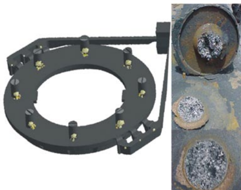
Fig. 5: Predicting shrinkage in cast iron components. Secondary shrinkage below risers is shown for a ductile iron ring casting. This confirms that a simple heat flow calculation is not sufficient, as it only shows a ring shaped temperature distribution in the center of the casting. Only the combination of local shrinking and expansion behavior leads to a correct defect prediction.
