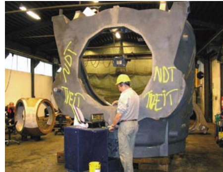
Fig. 21: Casting process simulation strongly supports the development of wind power casting technology. Compared to welded parts, castings offer much better fatigue properties, which is essential for components with a required minimum lifetime of 20 years. The weight of the castings is a critical factor for the functionality and price of a wind turbine. This means designer and foundry must strongly cooperate to take full advantage of the material performance for an optimized part. (*The picture is with friendly permission of Vestas, Norway)
