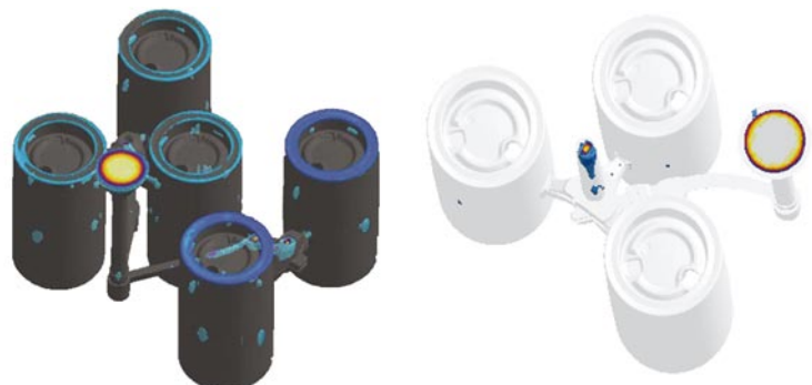
Fig. 7: Is a riser needed or not? The porosity prediction for an original riserless lay-out for a grey iron grade 250 casting shows problems near the top surface (left picture). The simulation clearly demonstrates the liquid shrinkage to be the root cause of the problem. Porosity prediction for a modified layout shows that a small riser completely compensates liquid shrinkage (right picture). (*The picture is with friendly courtesy of ITT Water and Wastewater AB)
