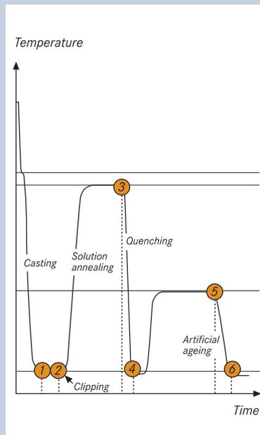
Temperature curve during the production chain of thin-walled structural castings
