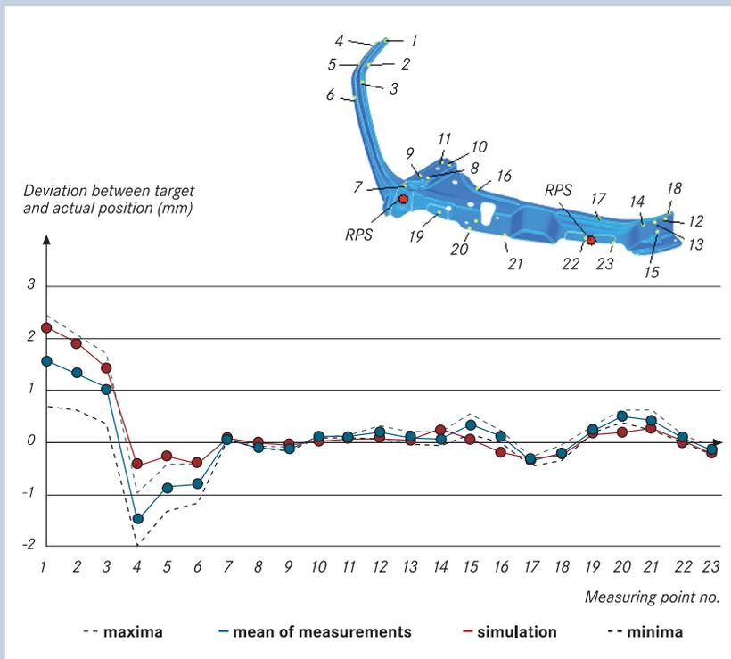
Calculated versus measured distortion after clipping
