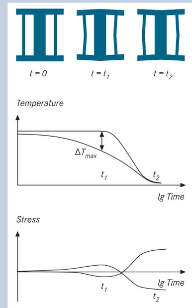
Underlying mechanism for the development of residual stresses and distortion by the example of a stress lattice
