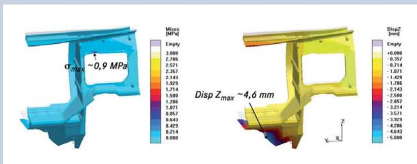
Stress distribution and deformation of the bulk head after solution annealing. The non-deformed bulk head geometry is shown transparent.
