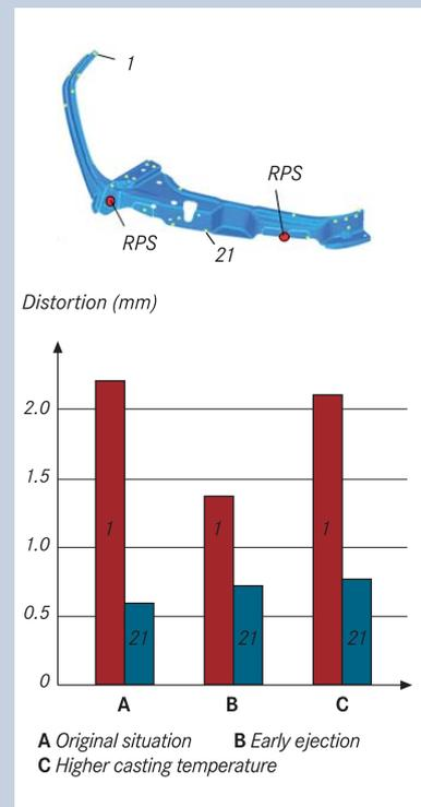
Parameter sensitivity of distortion calculated for the measuring points 1 and 21
