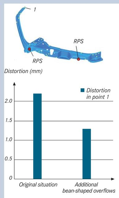
Effect of changed temperature distribution on the distortion of the "swan neck" after casting
