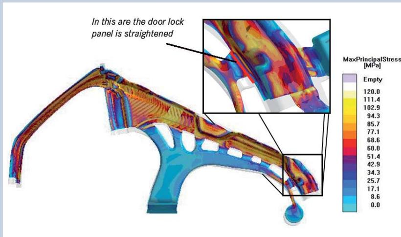
Maximal tensile stresses immediately before casting ejection. For illustration purposes the deformed and the non-deformed (transparent) geometries are shown.
