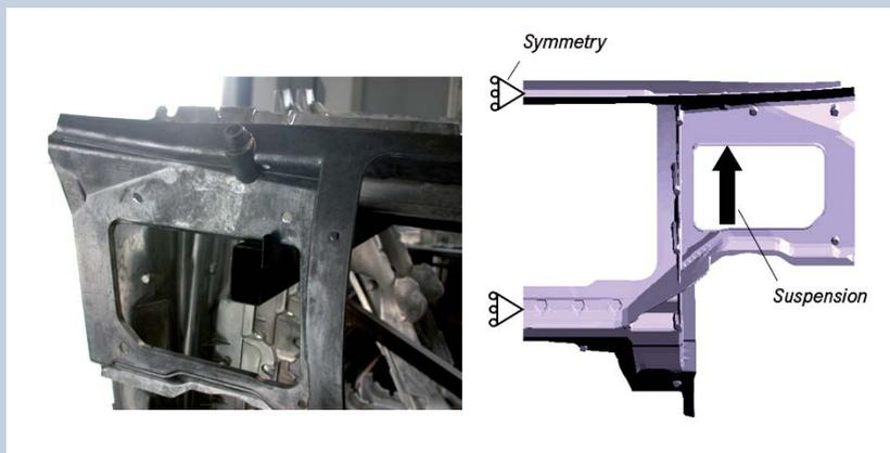
Suspension of the bulk head during heat treatment
